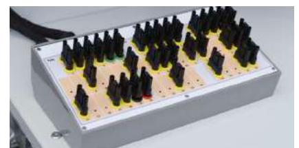
Interruption box control unit
