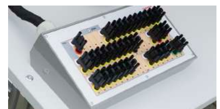
Interruption box control unit
